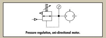
When both the speed and the torque are to be controlled the best configuration is to use a pressure regulator in the air line to the motor and a flow control valve on the outlet port. This way every point in the torque-speed graph can be set accurately.
