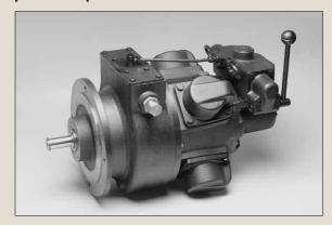
Radial Piston Air Motor Available with proportional hand or remotely controlled valve, pneumatic brake and all types of gearboxes. Power from 0,8 to 23 kW.
